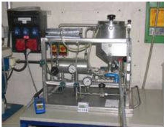
Figure 2. Bench-scale pressure-driven membrane system Memcell.
