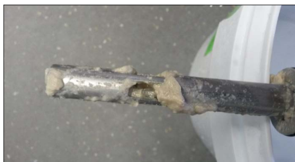
Figure 15. Probe fouling due to the filamentary structure of the fungi in a P. chrysogenum production process.
