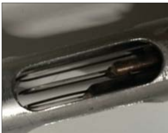
Figure 8. Picture of the probe, note the different length of the U-shaped wire sensors leads to different resonance frequencies for each sensor.
